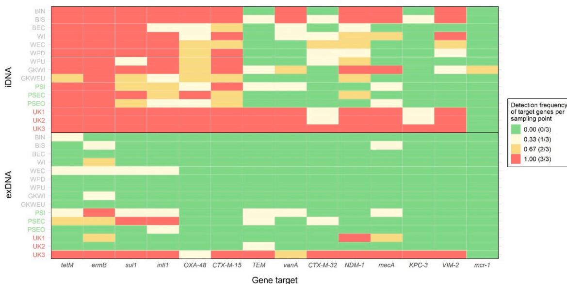
Fig. 4. Detection frequencies of target ARGs and intI1 at the examined sampling sites. Colours of the sampling point IDs represent municipal (grey), livestock (green) and clinical (red) wastewater. BIN, BIS, WI, GKWI: municipal influents; BEC, WEC: municipal effluents after conventional treatment; GKWEU: municipal effluents after ultrafiltration; PIS, PEC, PSEO: influents, effluents after biological treatment, and ozonation, respectively, from the on-site WWTP of the poultry slaughterhouse; UK1, UK2, UK3: clinical wastewater; WPU, WPD: pre-flooder of a municipal WWTP upstream and downstream of the discharge point, respectively.
