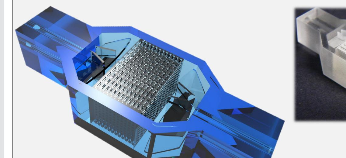
To meet the specific demands of the respective enzymes concerning optimal temperature, disposable reactor modules were designed, that can be individually heated.
