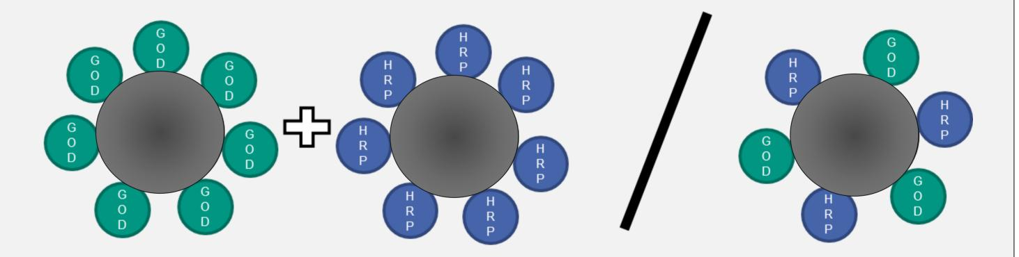
Approach III: Compartmentalized immobilization within temperature regulated reactor modules
