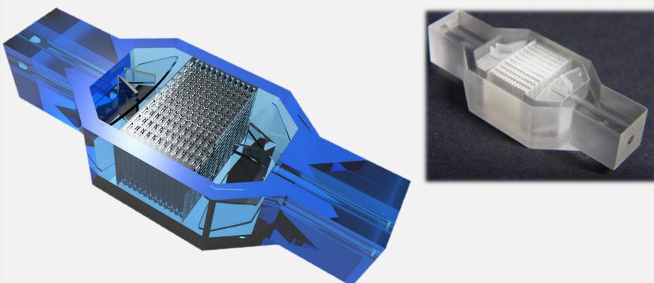
To meet the specific demands of the respective enzymes concerning optimal temperature, disposable reactor modules were designed, that can be individually heated.
