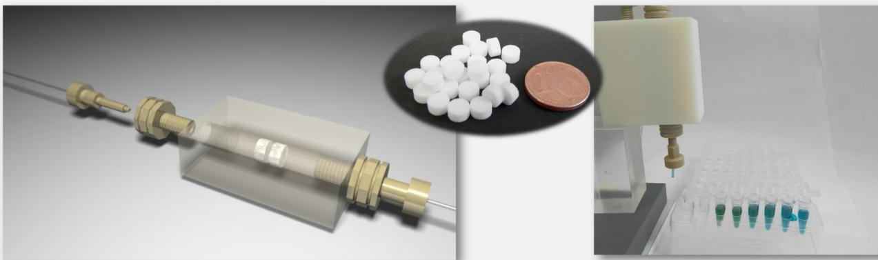
A reactor device for the perfusion of microfilters was designed and manufactured by 3D-printing.
